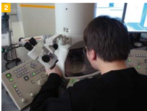
Figure 2: The research of the precipitations and their origins requires a transmission electron microscope (TEM) like the JEOL JEM-2100 being used. This TEM is equipped with the Cantega G2 by Olympus Soft Imaging Solutions (OSIS), a 2k x 2k TEM camera. For image acquisition and image analysis Artem Yurovskikh and colleagues use iTEM, the OSIS TEM imaging platform and iTEM Solution Diffraction.
